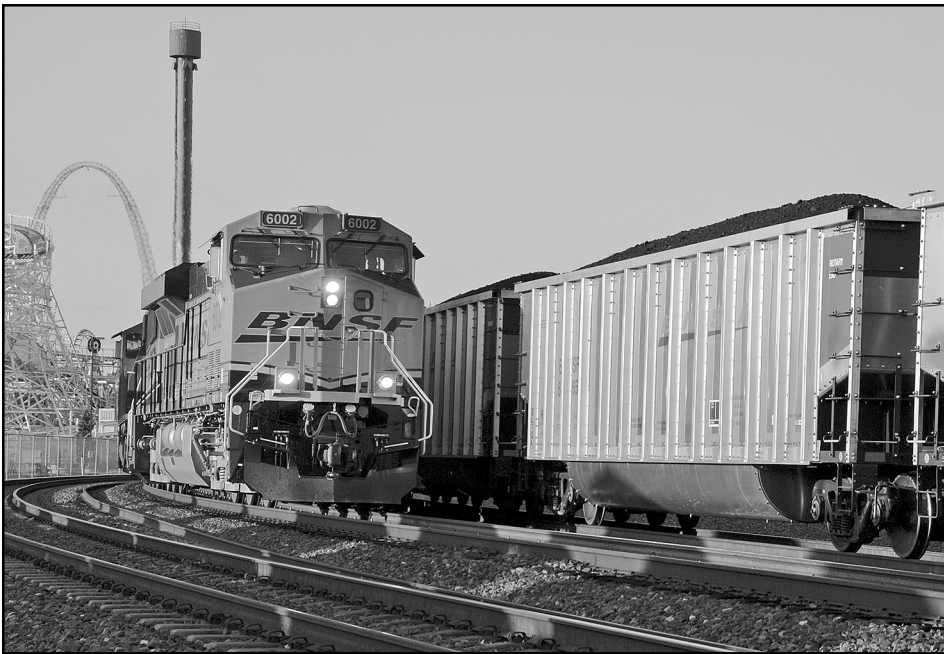
BNSF 6002 South passes new BNSF coal hoppers at LoDo Siding. BNSF's investment in new equipment for the Wyoming Southern Powder River Basin was apparent when new (delivered June 2006) BNSF ES44AC 6002 passed newly built BNSF aluminum hoppers on LoDo Siding in Denver on 9/12/06. The TriinityRail built hoppers had a builder's date of 08-06 (August 2006). – Photo © 2006 by Chip.
