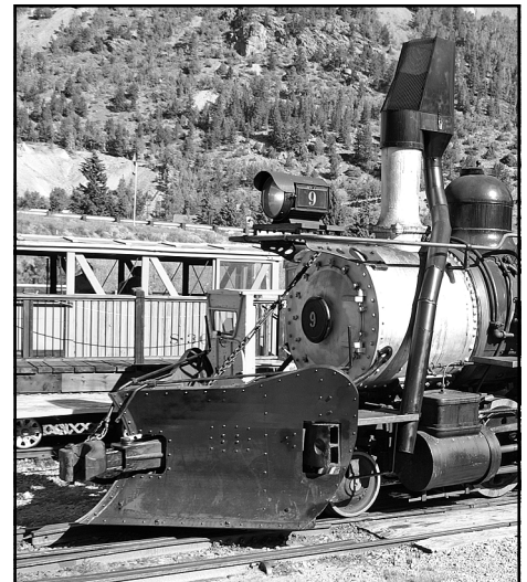
In the last week of August, the RailStar crew at the Georgetown Loop installed a new Ridgeway spark arrester on Colorado & Southern No. 9. Seen here on September 1st, the engine now has both a butterfly plow and the cinder catcher. –Photo © 2006 Dave Schaaf.
